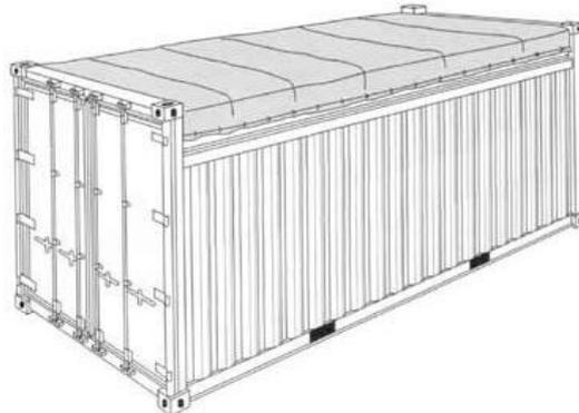
FIGURA 2.6 — ESQUEMA DE UM *CONTAINER OPEN TOP*
